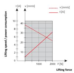
max. 2,000 N pressure max. 2,000 N tension 21 mm/s lifting speed max. up to 600 mm lift
