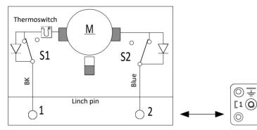
S1= Limit switch for traversing direction -extract-
