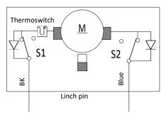
S1= Limit switch for traversing direction -extract-
