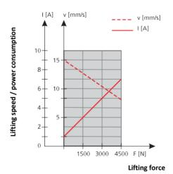
max. 4,500 N pressure max. 4,000 N tension 8 mm/s lifting speed max. up to 600 mm lift
