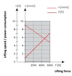
max. 6,000 N pressure max. 4,000 N tension 5 mm/s lifting speed max. up to 400 mm lift
