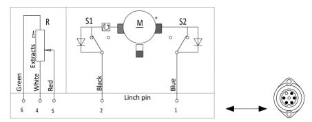
S1= Limit switch for traversing direction -extract-
